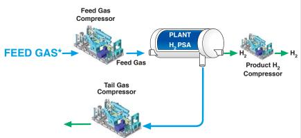
\* Feed Gas can be either **Syngas** coming from Reformer or Hydrotreater, or **Permeate Gas** coming from membrane plant
